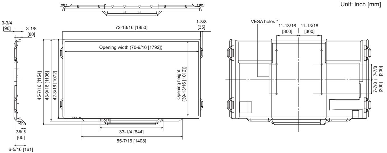
When mounting the monitor, be sure to use a wall-mount bracket that complies with the VESA-compatible mounting method. SHARP recommends using M6 screws and tighten the screws.
