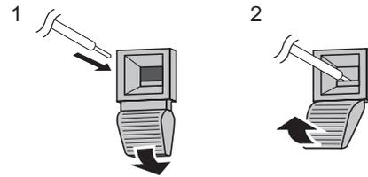
1. While pushing the tab, insert the tip of the cable.
