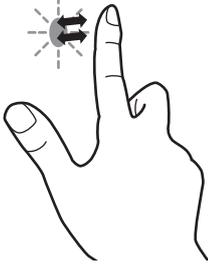
When double-tapping with your finger, be sure to lift your finger sufficiently off the screen after the first tap. If there is insufficient distance between the screen and your finger, double-tap will not take place.
