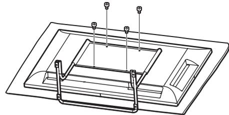
3. Reverse the stand assembly procedure to disassemble the stand.
