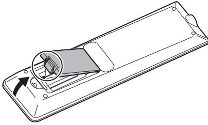
2. See the instructions in the compartment and put in the batteries (R-03 ("AAA" size) x 2) with their plus (+) and minus (-) sides oriented correctly.
