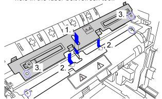
Fasten the fuser belt refresh tool to the machine with the screws that fastened the paper guide.
