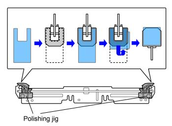
Adjust the positions of the fuser belt refresh tool polishing jigs to match the width of the paper where the lines appear.
