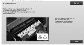
3) Replace the paper guide with the fuser belt refresh tool.
