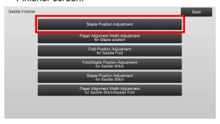
2) Adjust the staple positions in the direction of paper width.
