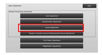
2) To print a test patch, tap the [Execute] key in the Density Smoothing Adjustment (Visual Adjustment) screen. If you need to change the density, select the desired density and then tap the [Execute] key.
