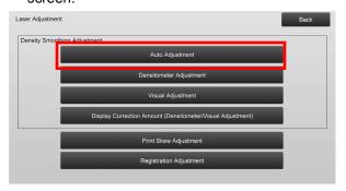
To print a test patch, tap the [Execute] key in the Density Smoothing Adjustment (Auto Adjustment) screen. If you need to change the density, select the desired density and then tap the [Execute] key.
