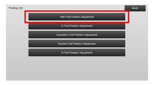
2) Adjust the saddle fold position for when the folding unit is installed.
