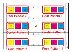
You can find the color image registration check patterns of two for front side, rear side and center each (total 6 places). Perform the adjustment by patterns visually. Horizontal direction is sub-scan direction (SUB) and vertical direction is main-scan direction in the above figure.
