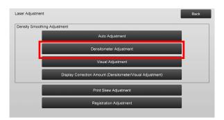
2) To print a test patch, tap the [Execute] key in the Density Smoothing Adjustment (Densitometer Adjustment) screen. If you need to change the density, select the desired density and then tap the [Execute] key.
