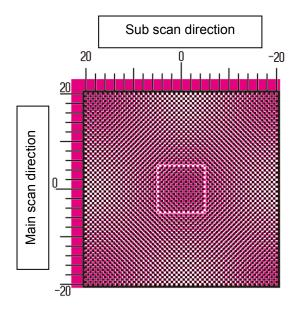
Perform adjustment so that the highest part in density around center of the check pattern fits within the adjustment standard frame for color registration at the center. Make sure to make the deviation at each pattern around the same level and minimize the entire deviation. Example:
