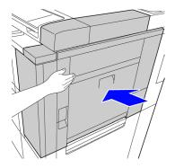
5) After replacing the paper guide with the fuser belt refresh tool, tap the [Next] key.
