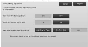
Main Scan Direction Adjustment: Select [ON] or [OFF]. Default: [ON]
