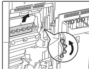
Rotate knob and remove the misfed paper.
