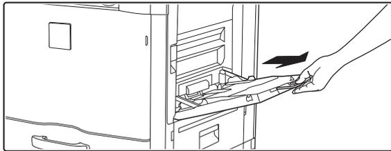
When loading a large sheet of paper, be sure to pull out the bypass tray extension. Pull the bypass tray extension all the way out.
