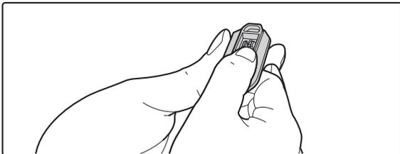
(2) Use your other hand to press down on the hook that secures the cleaner and remove the cleaner.
