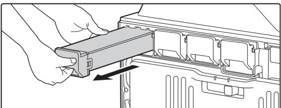
Hold the toner cartridge with both hands as shown and pull it out of the machine.
