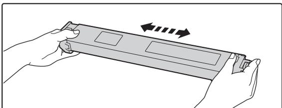
**Remove a new toner cartridge from its package and shake it horizontally five or six times.**
