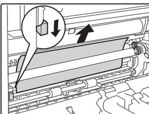
Lower the lever in the direction of the arrow to remove the misfed paper.
