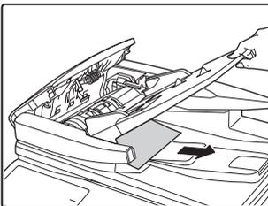
Pull out the document feeder tray and remove the misfed paper.
