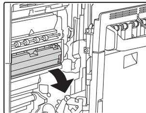
If the misfed paper is inside the fusing area, press down on the green part to tilt the fusing unit down toward you.
