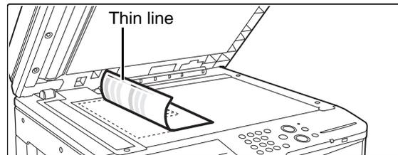
Lay copy paper (about five sheets) that is the same size as the test patch on top of the placed test patch, gently close the automatic document feeder, and touch the [Execute] key.
