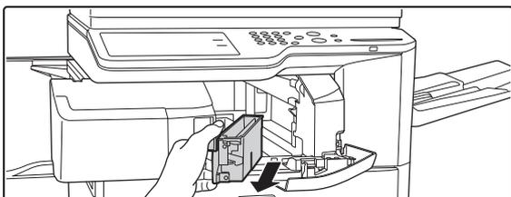
Grasp the punch waste box handle, gently pull out the box, and discard the punch waste.
