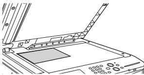
If the X dimension (width) of the document is less than 5-1/2" (140 mm) or the Y dimension (height) is less than 5-1/8" (131 mm), place the original on the document glass. For a thin original, use "Slow Scan Mode".
