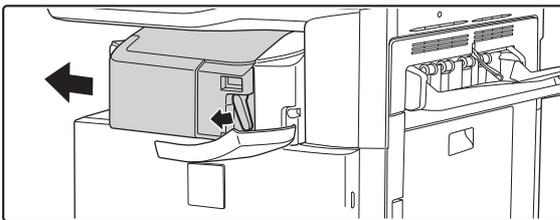
**While pressing the lever over to the left, slide the finisher to the left until it stops.**
