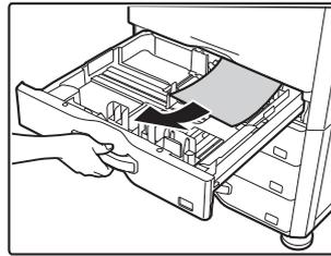
Before pulling the tray out, open the right cover and check if there is a paper misfeed. If you pull the tray out without checking, you may tear misfed paper and make it more difficult to remove the pieces that remain in the machine.
