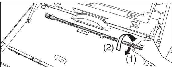
**Take out the cleaning tool for the laser unit.**
