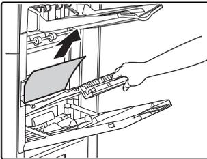
Open the Paper reversing section cover and remove the misfed paper.
