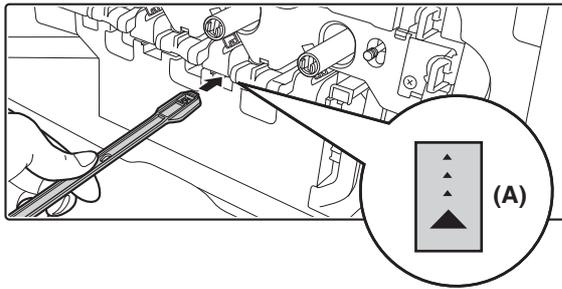
**Open the inner cover and clean the laser unit.**
