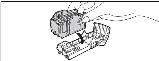
**Insert a new staple cartridge into the staple case as shown.**
