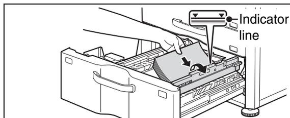
\*1 The paper stack must not be higher than the indicator line.
